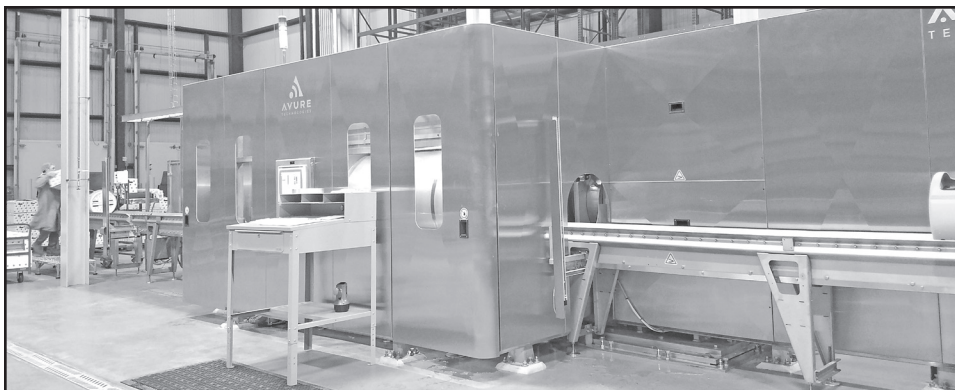
Hydrofresh HPP’s high pressure processing chamber
